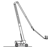
To remove the fault, move and hold the emergency power switch and activate the secondary boom up function until the secondary boom begins extending.
