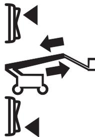
**27 Dual axis proportional control handle for primary boom up/down and turntable rotate left/right functions**
